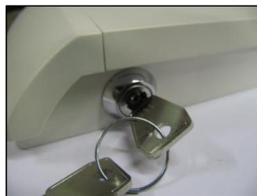
*Turn Anti-Clockwise to switch 'on'*
